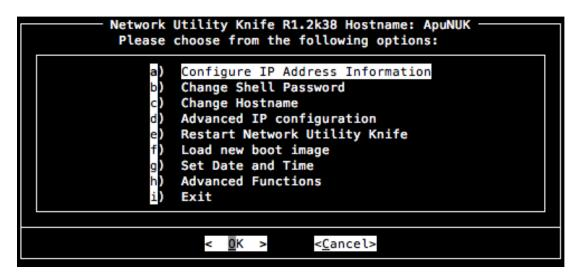
After logging in via SSH or the serial console, menu choice B allows you to change the SSH/serial console password.
