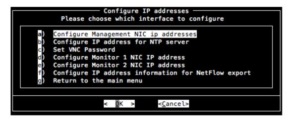
The change in IP address only takes effect after a reboot. If you want to test the IP address after a reboot, menu choice H, followed by menu choice A allows you to do a ping test. **Menu choice H** (from the main menu), also has **menu choice G** to check the ARP table).
